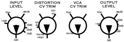
VCA CV TRIM might need adjustment to work properly with a given envelope generator. The VCA CV inputs can vary from -10v to +10v, although the usable range of the CV is about 0-4 volts for maximum gain variation. Again, the DISTORTION CV or control knob may be varied at the same time, to give sound variations that conventional VCA cannot.
