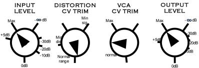
Input and output level should be set as needed, although maximizing both might be needed since variation of DISTORTION CV TRIM can also change the circuit gain considerably. The DISTORTION CV
