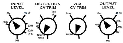
Note that the R-51 controls have considerable "extra range" beyond what they absolutely need. This is made necessary by variations in tube samples and to allow for tube aging. Do not assume these settings are written in stone, and if a different setting gives optimum results for your R-51, this is normal. Because the R-51 is totally different from any other synthesizer module you have ever used, you may be surprised by some of its quirks.
