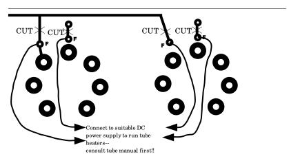
Note: this is an ADVANCED MODIFICATION and is NOT RECOMMENDED for inexperienced personnel. All R-series modules can be modified to accept +-15v power supply rails and MOTM-standard power connectors. The user is responsible for fabricating a suitable front panel and adding controls and jacks as needed for a given modular-synth form factor. Addition of two 20-ohm 2W dropping resistors and a 4-pin connector is involved. Contact us for more information on this modification.
