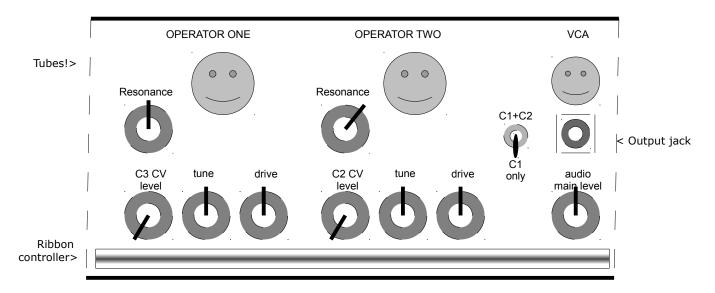
The path is very simple: operator one feeds directly into operator two, which feeds directly into the VCA.
