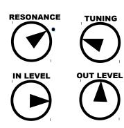
The dot next to the RESONANCE knob indicates where the best setting is for low-distortion sine wave
